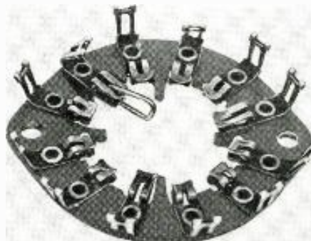
Fig. 2—Wire placed in contact groove keeps it from getting deformed during repair.
