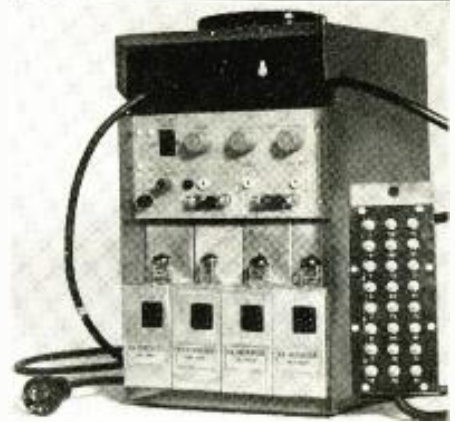
A package unit of four Hallamore Electronics negative-impedance repeaters complete with power supply.
