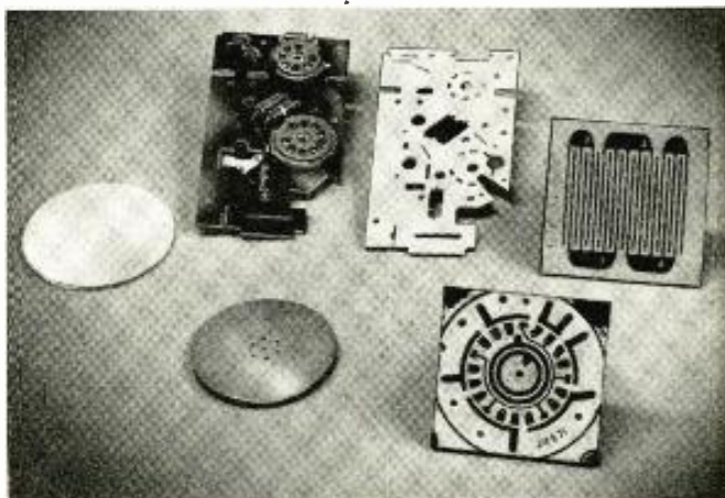
Fig. 10—A group of printed-circuit boards with ceramic bases. They are designed to withstand high temperatures.
