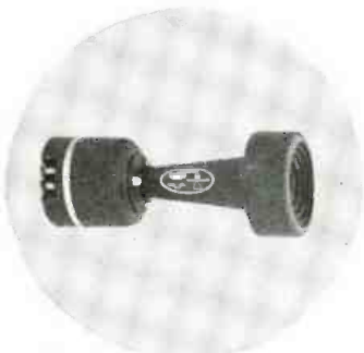
A high frequency assembly frequently used with the JBL D130 is the 175DLH consisting of a 1200 cycle crossover driver, exponential horn, and 90° projection-angle acoustical lens.
