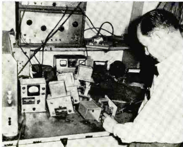
Murray Barlowe doing final assembly work on several of the electronic molten-glass level controls which he developed for a local plant of the Pittsburgh Plate Glass Co. in the course of servicing some of their control equipment.
